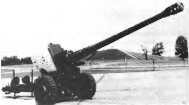
Figure 6-26. 122-mm field gun D-74. The D-74, with a range of about 23,900 m, can be rapidly shifted through a 360 degree traverse with the aid of a firing jack and the two large castor wheels on the trail.
